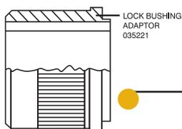
Recommended diameter of hole in mild steel fixture plate 25.4 mm / 25.43 mm to give press fit with lock bushing. For other fixture plate materials, hole diameter will vary.
