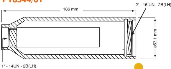
**Note: With longest nose housing PT8544/61 fitted max usable stroke is 54 mm**
